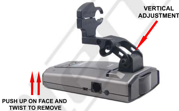
6 - Install the RD onto the mount. Make necessary adjustments using the upper and lower pivots, and the vertical adjustment. Leave enough room below bottom of mirror to allow access to top radar detector buttons. To remove the radar from the magnetic mount, simply tilt the face of the RD up and twist slightly to side, then the magnet will release.
